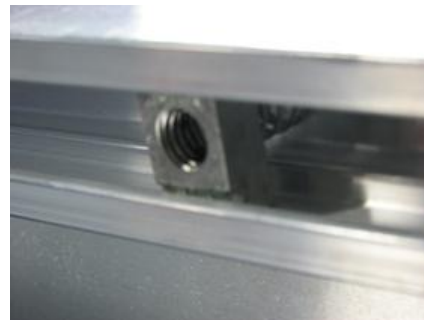
Correct spring nut position
