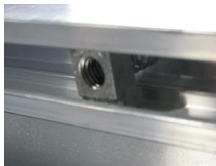
Correct spring nut position
