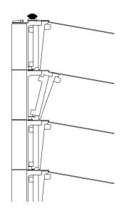
TILT LENS, SET BEHIND LOUVER OFFSET, AND SNAP UP INTO THE VERTICAL POSITION. LENS MUST BE SNAPPED UP IN AND BEHIND UPPER LOUVER OFFSET.
