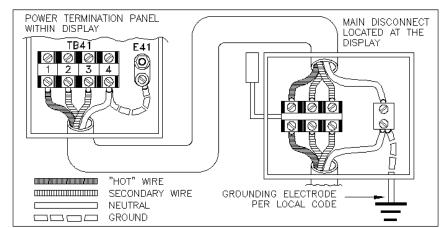
Figure 4: Installation with Only Neutral Provided
