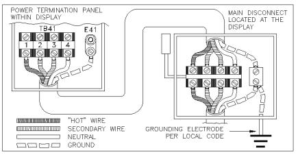
Figure 3: Installation with Ground and Neutral Provided
