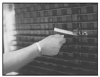
Figure 6: Removing a Module
