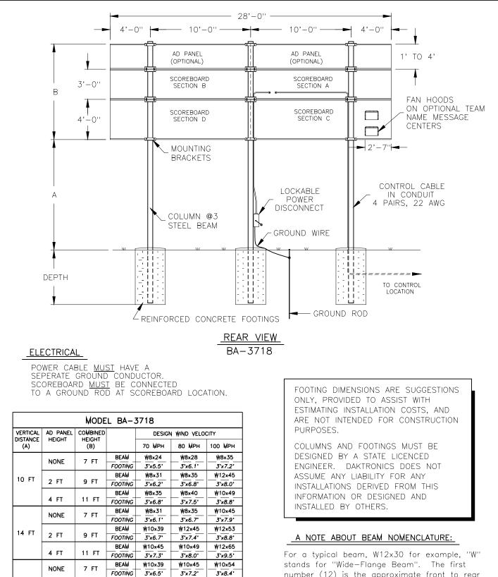
stands for "Wide-Flange Beam". The first number (12) is the approximate front to rear dimension of the beam in inches. The second number (30) is the weight per foot in pounds. This numbering is standard in the steel industry. Widths vary from 4 to 8 inches in this chart.
