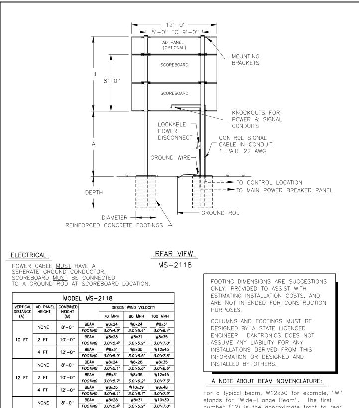
number (12) is the approximate front to rear dimension of the beam in inches. The second number (30) is the weight per foot in pounds. This numbering is standard in the steel industry. Widths vary from 4 to 8 inches in this chart.
