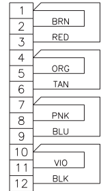
ADDRESS PLUG WIRE SIDE
