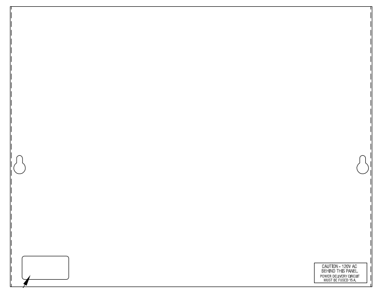
COVER, FRONT VIEW APPLY THE CAUTION 120V LABEL TO THE FRONT OF THE COVER, DOWN IN THE CORNER.
