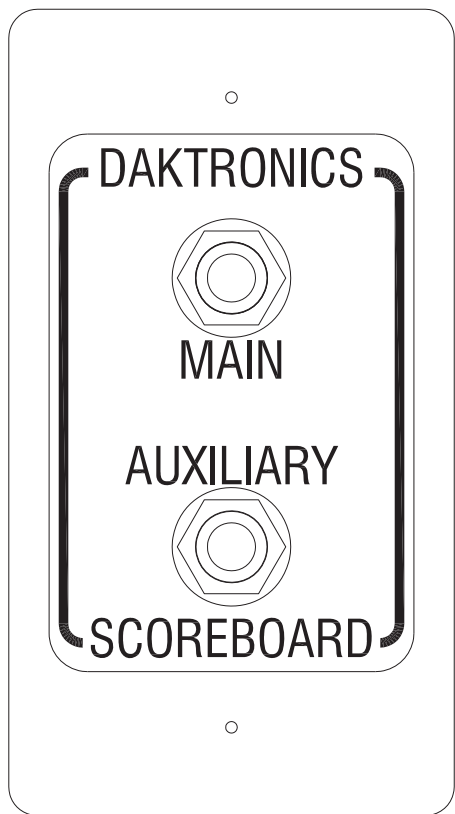
SCHEMATIC AUXILIARY 1/4" PHONE JACK
