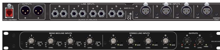
Figure 15: Part #: A-1960 Microphone/line mixer, front and back view
