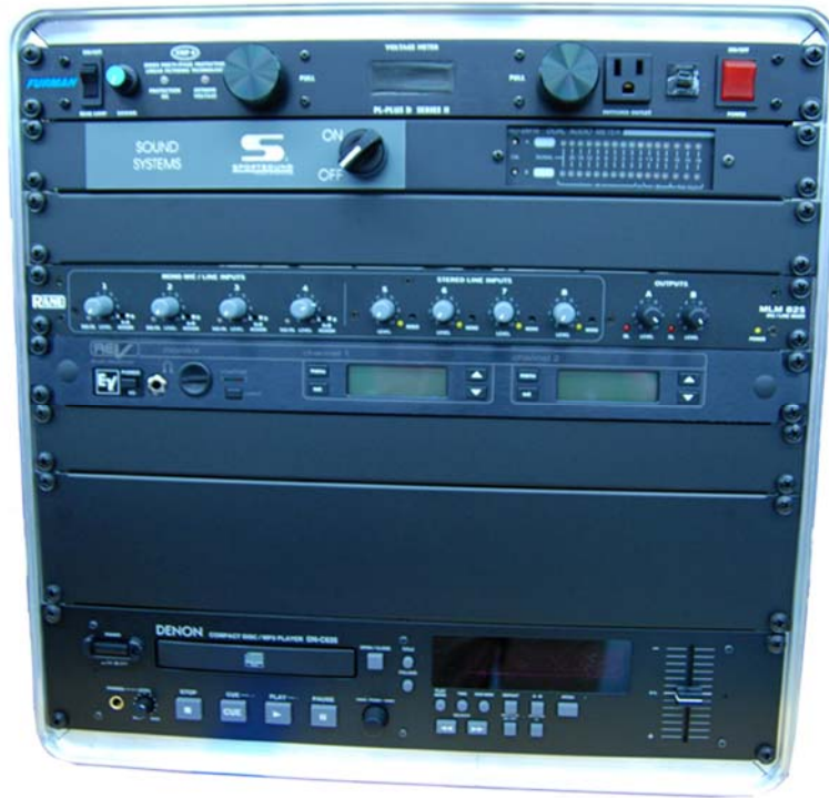
Figure 8: Portable announcer's rack
