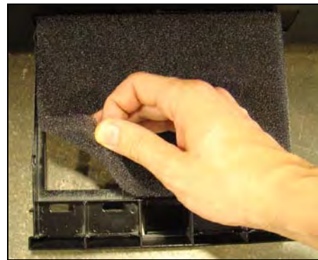
Figure 19: Removing Filter Medium
