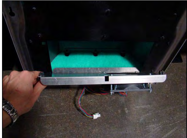
Figure 27: Removing Fan Assembly
