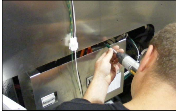
Figure 9: Removing Term Panel Support Screws
