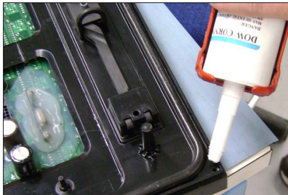
Figure 15: Fill in 23 mm Weep Holes
