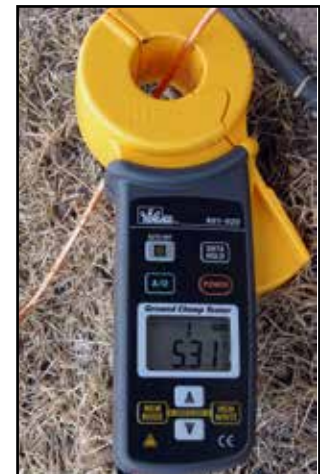
Figure 8: Measure Resistance to Ground
