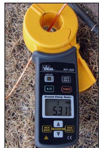
Figure 12: Measure Resistance to Ground
