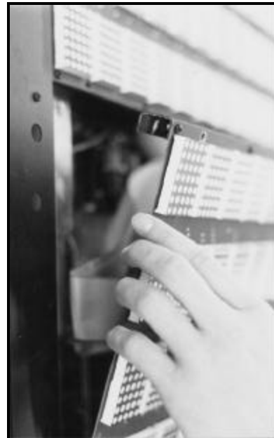
Figure 24: Removing LED Module Panel (1.2" & 2.1")
