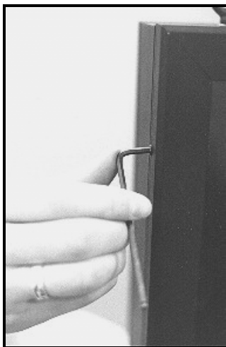
Figure 19: Removing the Face Panel Screws
