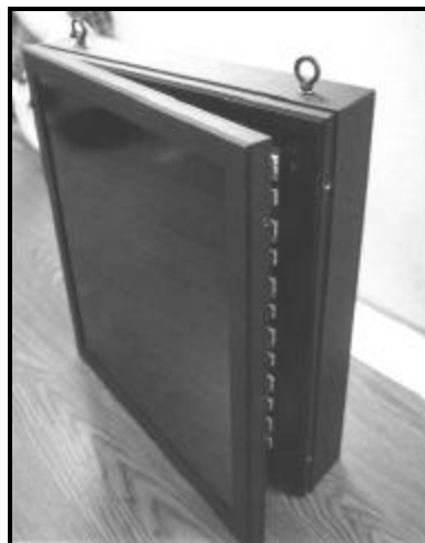
Figure 20: Face Panel Partially Removed
