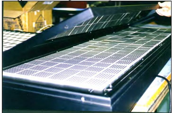
Figure 28: Display, Face Panel partially removed
