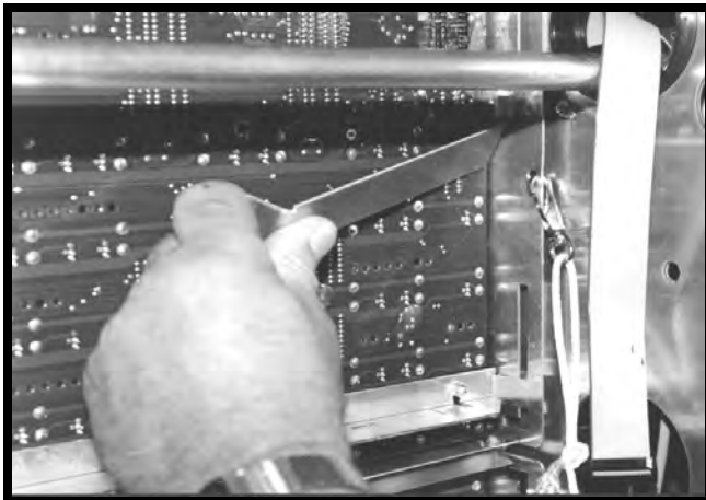
Figure 43: Inserting the Tool to Release the Lens Assembly Retaining Latch.
