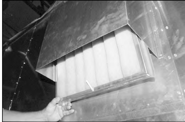
Figure 52: Filter Removal - Rear Access
